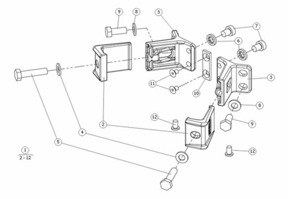
Spare Part C500 Screw kit seat elevator
